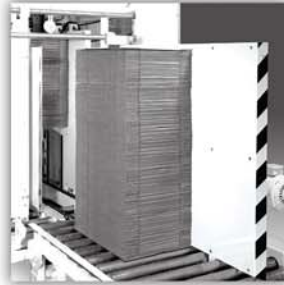
Stack of KD cases entering the FF 100 elevator
